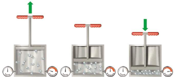
Lifting the plunger decreases the pressure of the gas. The particles of gas collide less often with the walls of the piston as they spread farther apart. The volume of the gas increases as the pressure decreases.
